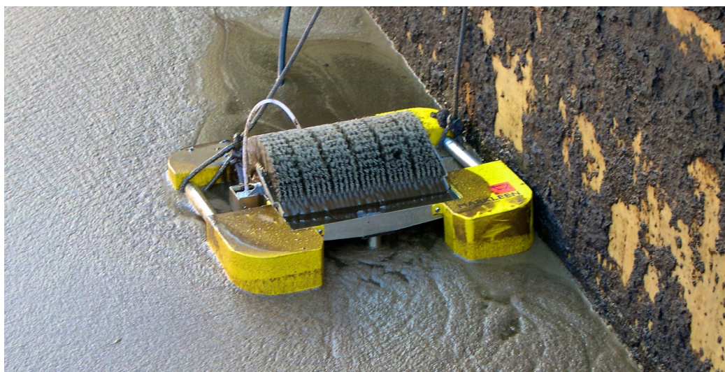
Figure 13: Brush skimmer in action
