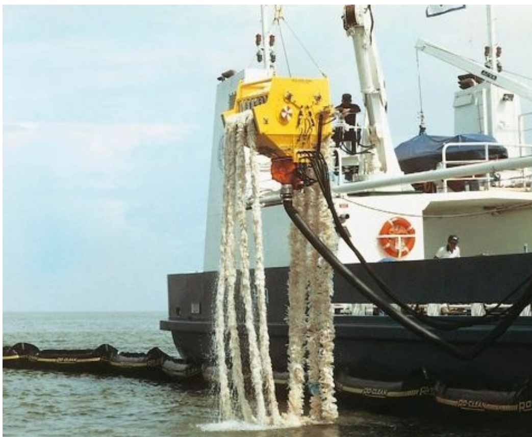
Figure 11: Rope mop skimmer in action
