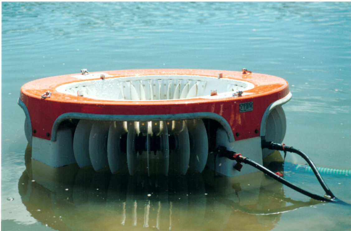
Figure 7: Disc skimmer in action
