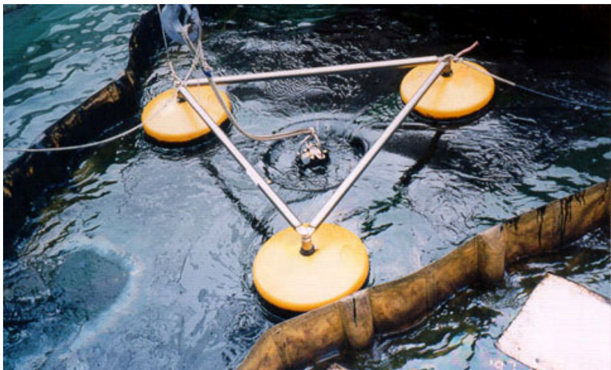
Figure 5: weir skimmer in action
